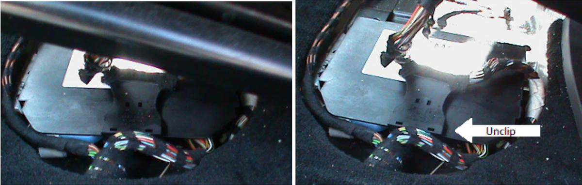
5. To release the module remove the plastic phillips head screw on the left side of the module
