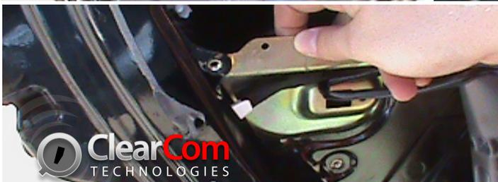
11. Look inside the door frame and remove the black clip attached to the bottom of the outer door handle
