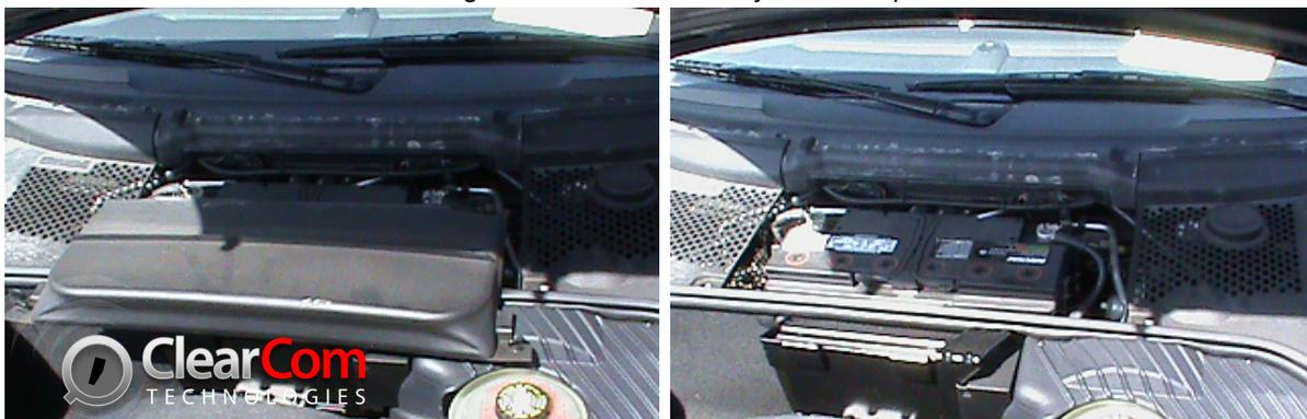
4. Lift the seat up and rest it on the small back seat. The alarm module should now be exposed
