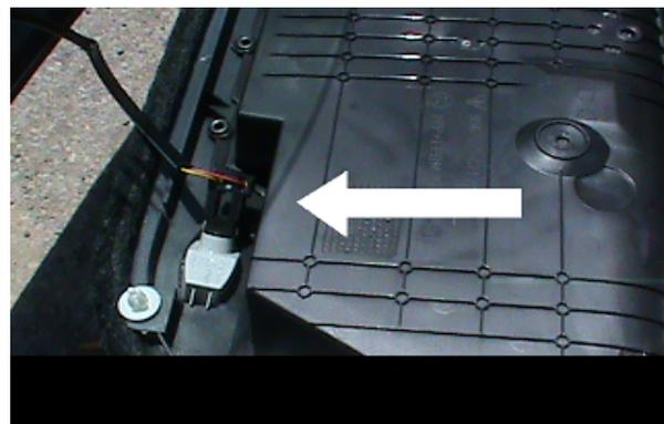
8. To remove the inner door handle cable pull out on the 2 plastic tails and push the clip left
