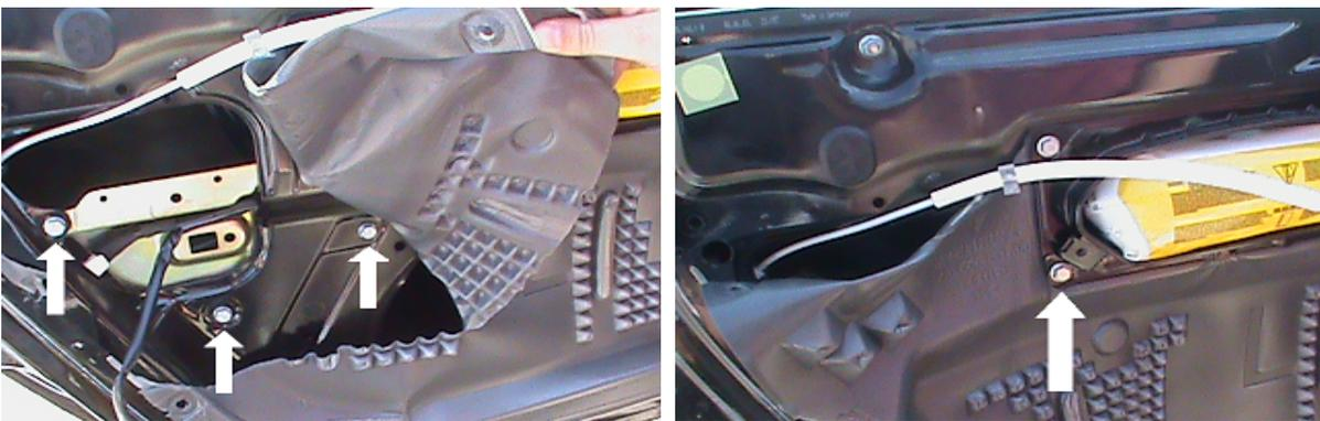
Now simply push the support bracket down inside the door frame and out of the way for easier access to the door lock
