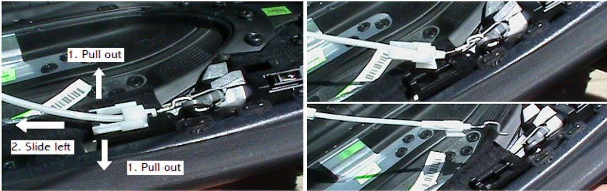
9. To access the door lock remove the gray clip holding the cable and wire
