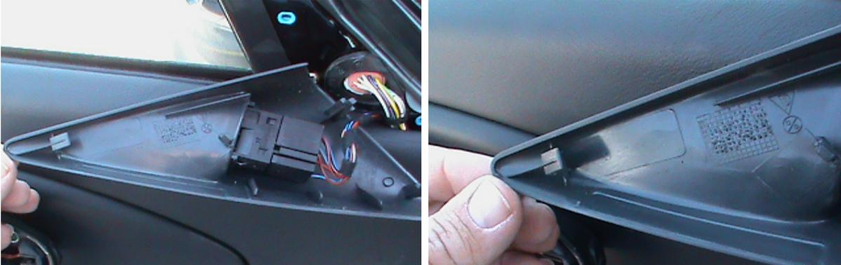
6. With the bolts, screws and mirror panel removed the door panel can be removed by popping the plastic clips on the outer edges of the panel and sliding it up off of the window frame.
