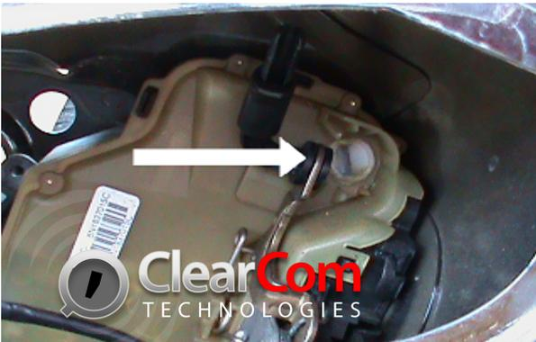
This is the slot in the latch that the tailpiece of the lock slides into.
